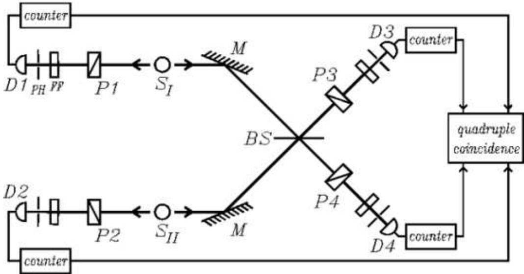
FIG. 6: Figure taken from Pavičić and Summhammer (1994): “Two photons from different unpolarised sources each pass through a polariser to a detector. Although their trajectories never mix or cross they exhibit 4th-order-interference-like correlations when the other two photons interfere on a beam splitter even when the latter two do not pass any polarisers at all.” [5]
