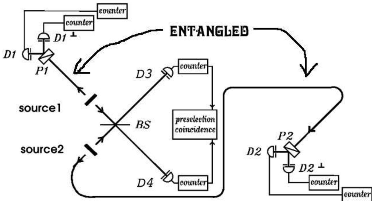
FIG. 7: Figure taken from Pavičić (1995): “In the experiment two photons from two singlets interfere at a beam splitter, and as a result the other two photons—which nowhere interacted and whose paths nowhere crossed—exhibit a 100% correlation in polarisation, even when no polarisation has been measured in the first two photons.” [17]
