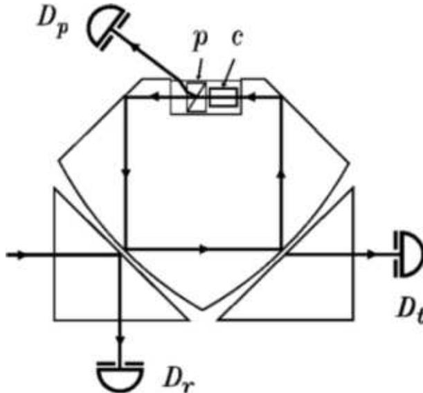
FIG. 5: Figure taken from Paul and Pavičić (1997): “Lay-out of the proposed virtual-or-real-path experiment. When the Pockels cell  $c$  is *on* it redirects the round-trip path through Rochon prism  $p$  into detector  $D_p$  and therefore almost only detector  $D_r$  fires. When the Pockels cell  $c$  is *off* there is no influence on the round-trip path and almost only detector  $D_t$  fires. [5]
