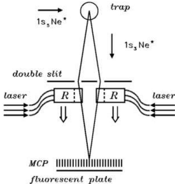
FIG. 4: Figure taken from Pavičić (1996): Proposal for a *welcher Weg* experiment with ultracold atoms. MOTIRR resonators R, see Fig. 2, here shown sideways, move together with the falling atoms which sit in their openings.” [7]
