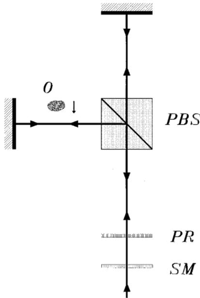
Fig. 3. Figure according to Ref. 7. A single horizontally polarized photon enters the resonator through the switchable mirror *SM* and passes the polarization rotator *PR* (which turns the polarization plane by the angle  $90^\circ/N$ ) and the polarizing beam splitter *PBS*  $N$  times before exiting through *SM* horizontally polarized when there is an object in the path and vertically polarized when there is no object in the path.
