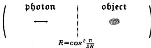
Fig. 2. Figure according to Ref. 4. A single photon inserted into the left cavity stays there when there is an object in the right cavity and moves to the right cavity when there is no object there.
