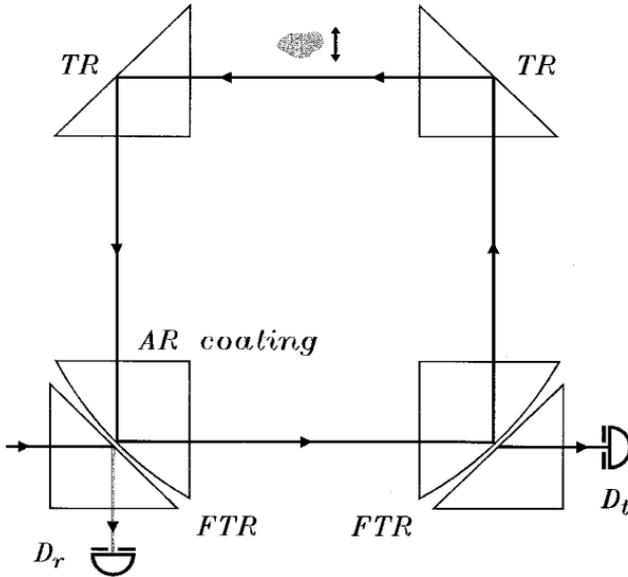
Fig. 4. Schematic of the proposed realistic interaction-free device. A single p-polarized photon tunnels (frustrated total reflection *FTR*) into the resonator. With a realistic efficiency exceeding 98% the beam makes several hundred loops guided by two total reflections *TR* and two *FTR*'s to exit into  $D_t$  when there is no object in the path. When there is an object in the resonator, the beam is reflected into  $D_r$ .
