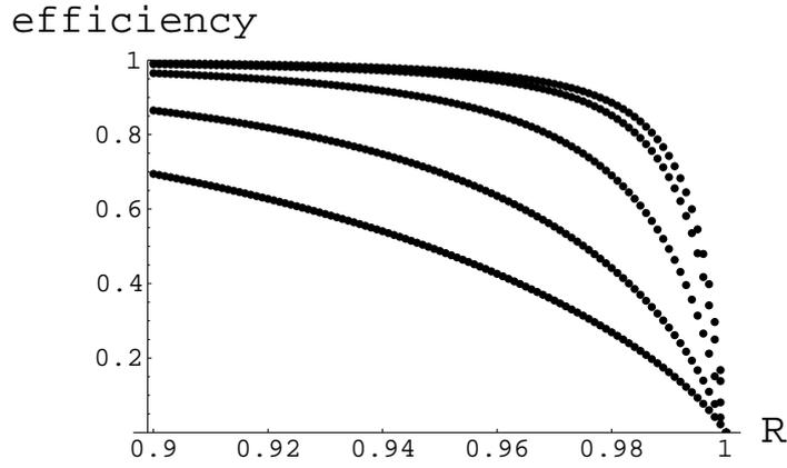
**Figure 5.**  $\eta$  as a function of  $a$ , the ratio of coherence time and the round-tip time for  $\rho = 0.99$  and  $0.9 \leq R \leq 1$ .  $a = 500$  (top), 150, 50, 20, and 10 (bottom).
