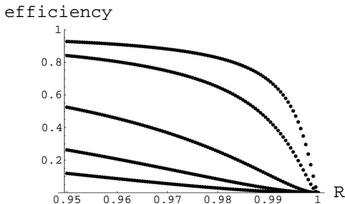
**Figure 4.** The efficiency of the throughput into  $D_t$  when there is no object in the resonator,  $\tau$ . We again have  $\rho = 0.998$  (top), 0.99, 0.98, 0.95, and 0.9 (bottom).
