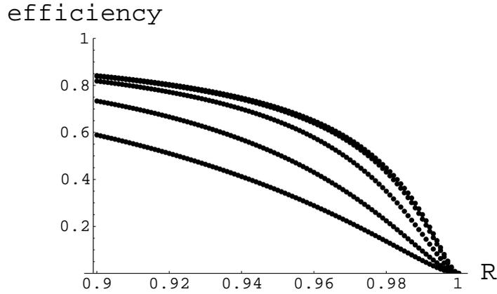
**Figure 6.**  $\tau$  as a function of  $a$  for  $\rho = 0.99$  and  $0.9 \leq R \leq 1$ .  $a = 500$  (top), 150, 50, 20, and 10 (bottom).
