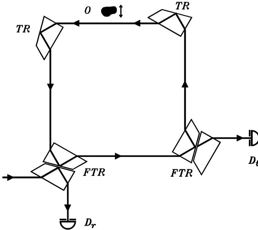
**Figure 2.** Schematic of the proposed realistic interaction-free device. A single p-polarized photon tunnels (frustrated total reflection) into the resonator made of Pellin-Broca prisms. With a realistic efficiency of over 98% the beam is guided by two total reflections and two frustrated total reflections to exit into  $D_t$  when there is no object in the path and is being reflected into  $D_r$  when there is.
