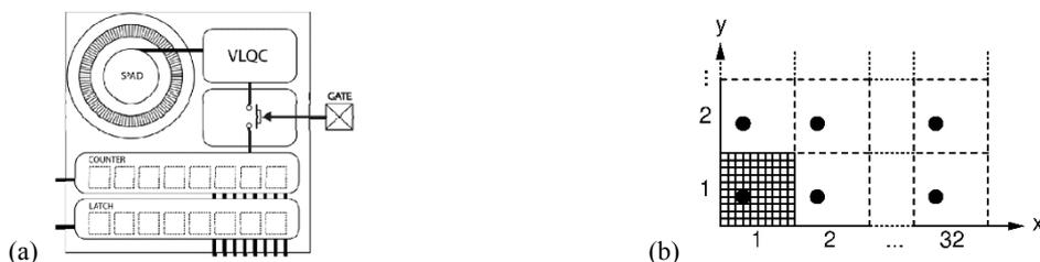
Figure 4. (a) Footprint of a single pixel cell in SPC2 (reprinted from [13] with the permission from MPD), (b) schematic diagram of camera walk in  $x$ - $y$  plane.
