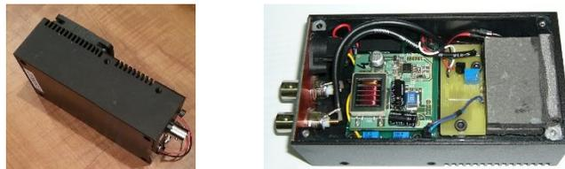
Figure 3. Photon-counting detector used for recording digital holograms with low light levels.
