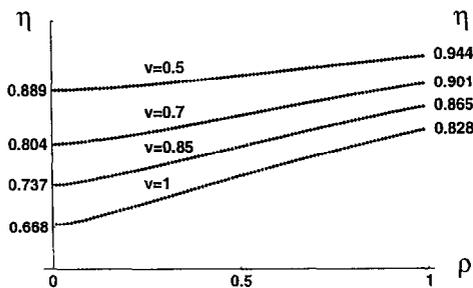
Fig. 2. Minimal detection efficiencies  $\eta$  necessary for violation of the Bell-Clauser-Horne inequality as functions of visibility  $v$  and of  $\rho = R/(1-R)$ , where  $R$  is the reflectivity of the beam splitter.
