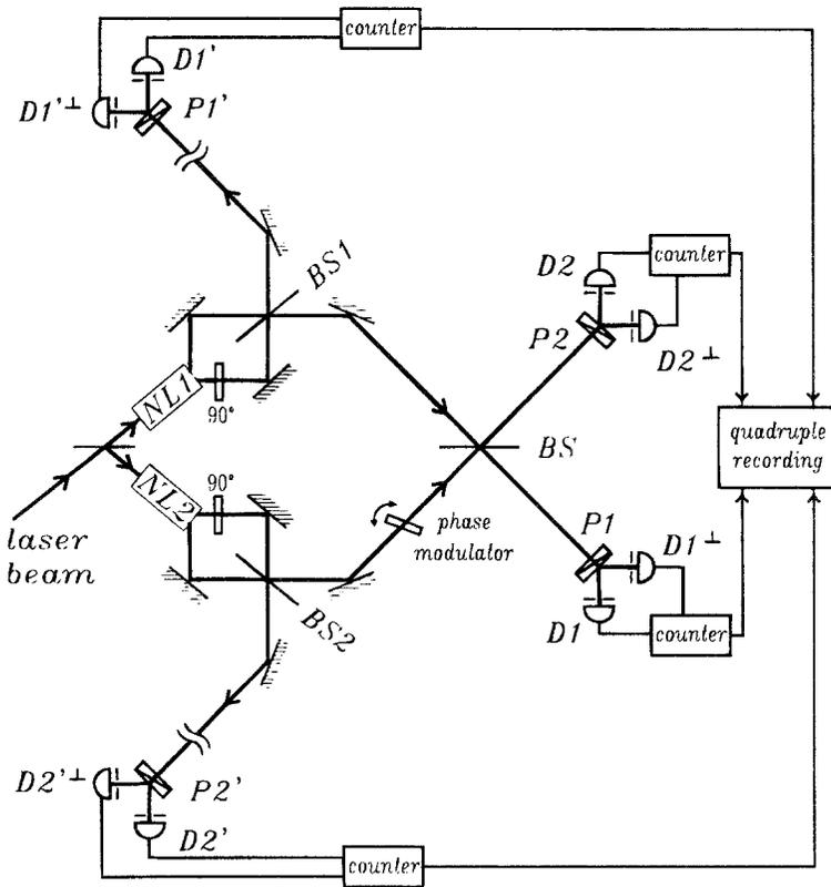
Fig. 2. Outline of the experiment. Distances between BS1 (BS2) and D1' (D2') in the experiment are assumed to be much larger than distances between BS1 (BS2) and D1 (D2) as indicated by the wavy lines.
