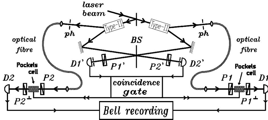
Figure 1: Lay-out of the proposed experiment. As the event-ready preselector serves a beam splitter with detectors  $D1'$  and  $D2'$  and their counters which open the gate (Pockells cells) for Bell pairs.
