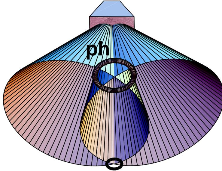
Figure 2: Photons from the cones are mutually perpendicularly polarized and therefore the photons from the intersections of the cones are in a singlet-like state. We chose pinhole  $ph$  five times bigger than the other one (determined by detectors  $D1'$  and  $D2'$ ) so that for each photon which passed through the latter pinhole, its *companion* photon will pass through  $ph$ .
